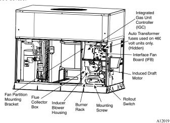
Fig. 21 – Blower Housing and Flue Collector Box
