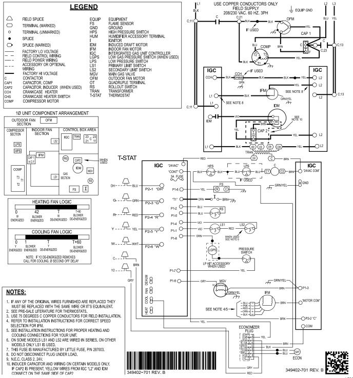
Fig. 19 – 460-3-60 Ladder Wiring Diagram
