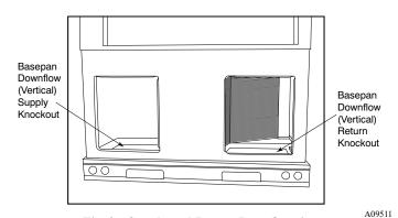
Fig. 9 - Supply and Return Duct Opening
