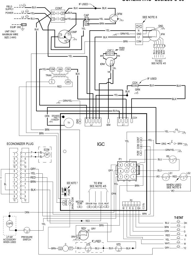
Fig. 16 – 208/230-3-60 Connection Wiring Diagram
