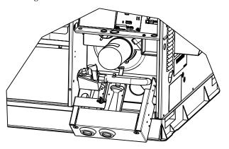
Fig. 24 - Burner Rack Removed
