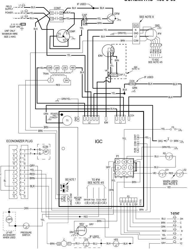
Fig. 18 – 460-3-60 Connection Wiring Diagram
