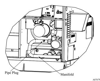
Fig. 11 - Burner Assembly
