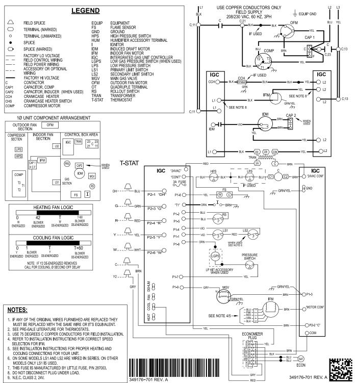
Fig. 17 - 208/230-3-60 Ladder Wiring Diagram
