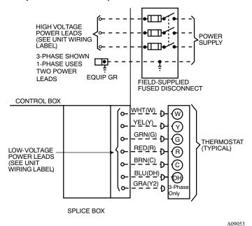
Fig. 10 – High- and Control-Voltage Connections
