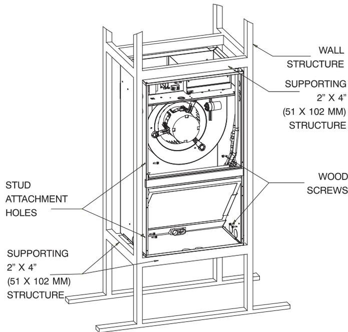
**Fig. 4 – Frame Mount Installation**
