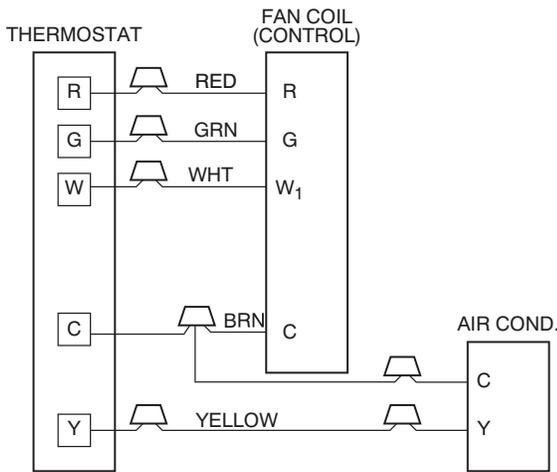
**Fig. 6 – Wiring Layout Air Conditioning Unit (Cooling and 1-Stage Heat)**
