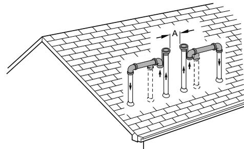
Fig. 47 – Pipe Vent and Combustion Ventilated Combustion Air A96128
