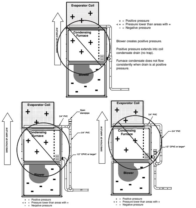
Fig. 13 – Example of Field Drain Attachment (Not Allowed)
