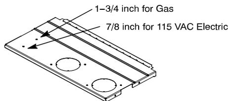
**Fig. 31 – Alternate Gas and Electric Entry**
