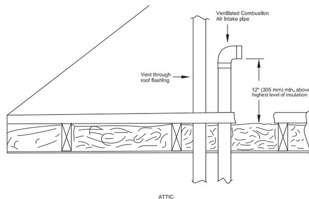
**Fig. 49 – Vent Terminations for Ventilated Combustion Air**
