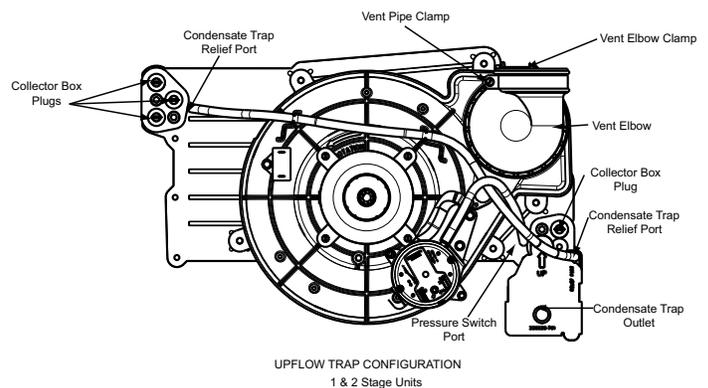
**Fig. 8 – Upflow Trap Configuration**
