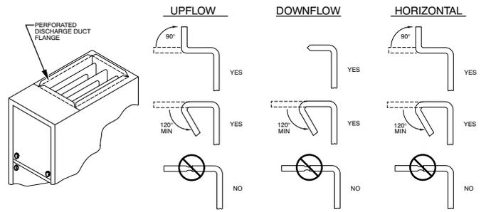
Fig. 20 – Duct Flanges
