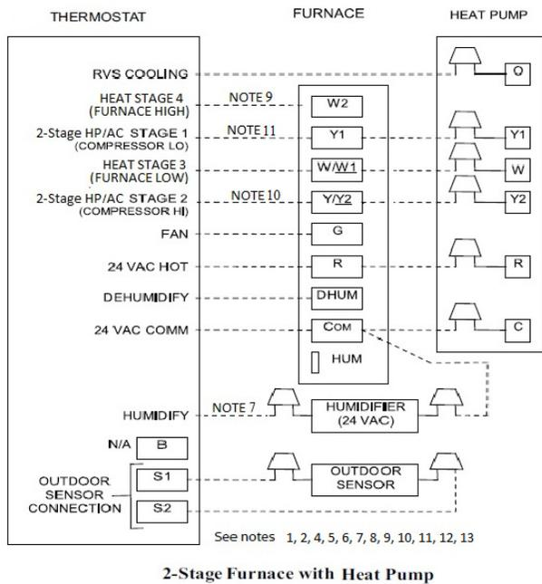
**Fig. 40 – Thermostat Connection for Two-Stage Furnace and A/C & Heat Pump**
