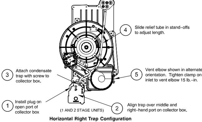
**Fig. 10 – Horizontal Right Trap Configuration
