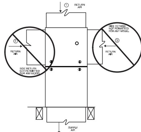
Fig. 22 – Downflow Return Air Configurations and Restrictions
