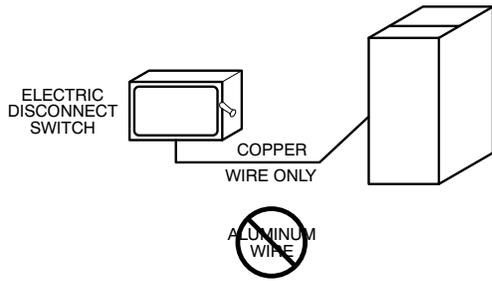
Fig. 33 – Field-Supplied External Electrical Box on Furnace Casing
