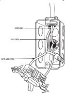
**Fig. 36 – Field-Supplied External Electrical Box on Furnace Casing NOTE:** If electrical entry through the furnace top panel is used, a 7/8-in. (22 mm) hole must be drilled through the top panel.
