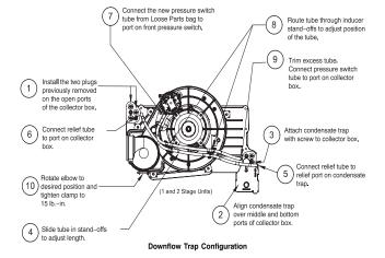
Fig. 9 – Downflow Trap Configuration
