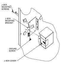
Fig. 35 – Installing J-Box (When Used)
