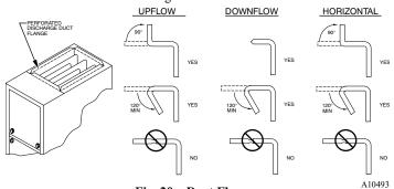
Fig. 20 - Duct Flanges
