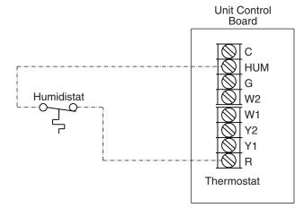
Fig. 37 — Humidistat Connections to UCB
