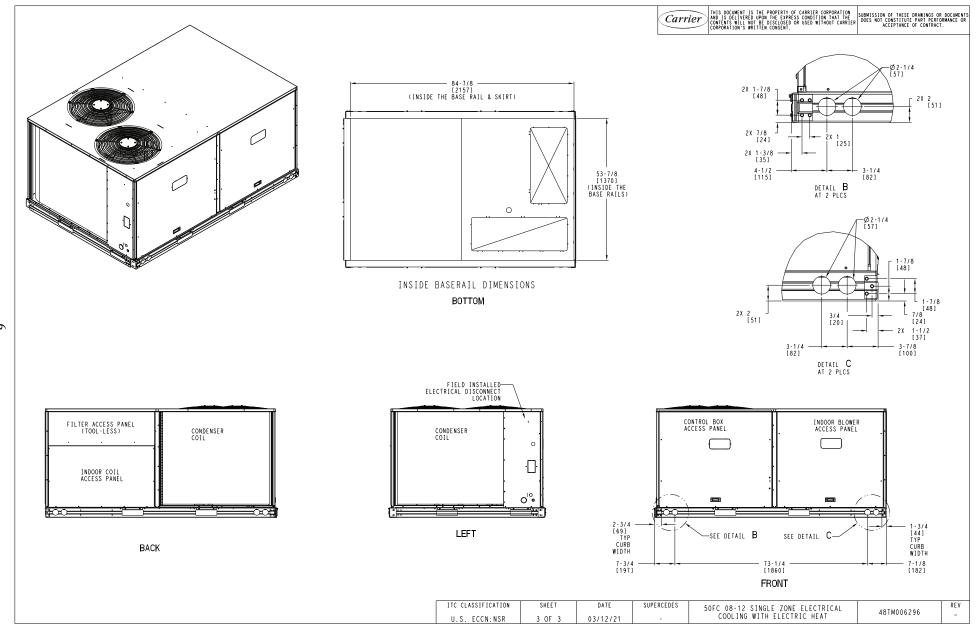
Fig. 2 — 50FC 08-12 Unit Dimensional Drawing (cont)
