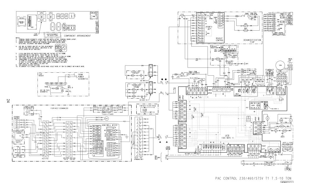
Fig. 39 — Typical Control Wiring Diagram, Electro-Mechanical with W7220 (50FC 08-12 230/460/575-3-60 Unit Shown)
