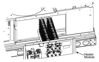
Fig. 32 — Typical Heater Module Installation
