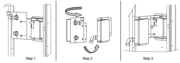
Fig. 51 — Completing Installation of Return Air Smoke Sensor
