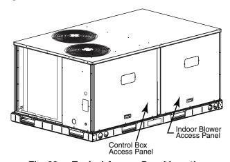
Fig. 30 — Typical Access Panel Location
