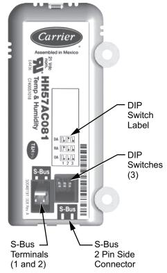
Fig. 46 — S-Bus Sensor DIP Switches
