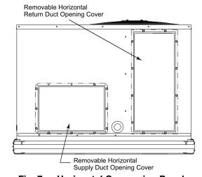
Fig. 7 — Horizontal Conversion Panels
