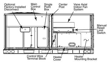
Fig. 31 — Typical Component Location
