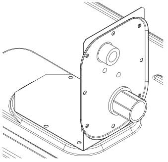
Fig. 26 — Thru-the-Base Fitting Assembly (Shown in Shipping Position)
