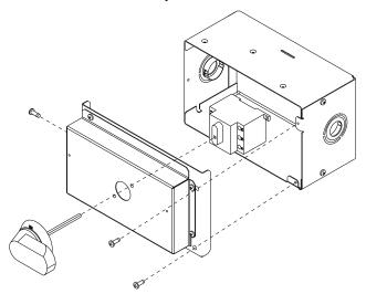
Fig. 20 — NFD Handle and Shaft Assembly
