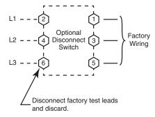
Fig. 17 — Power Wiring Connections
