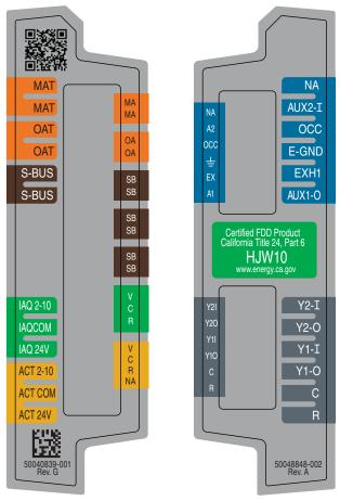
Fig. 45 — W7220 Wiring Terminals
