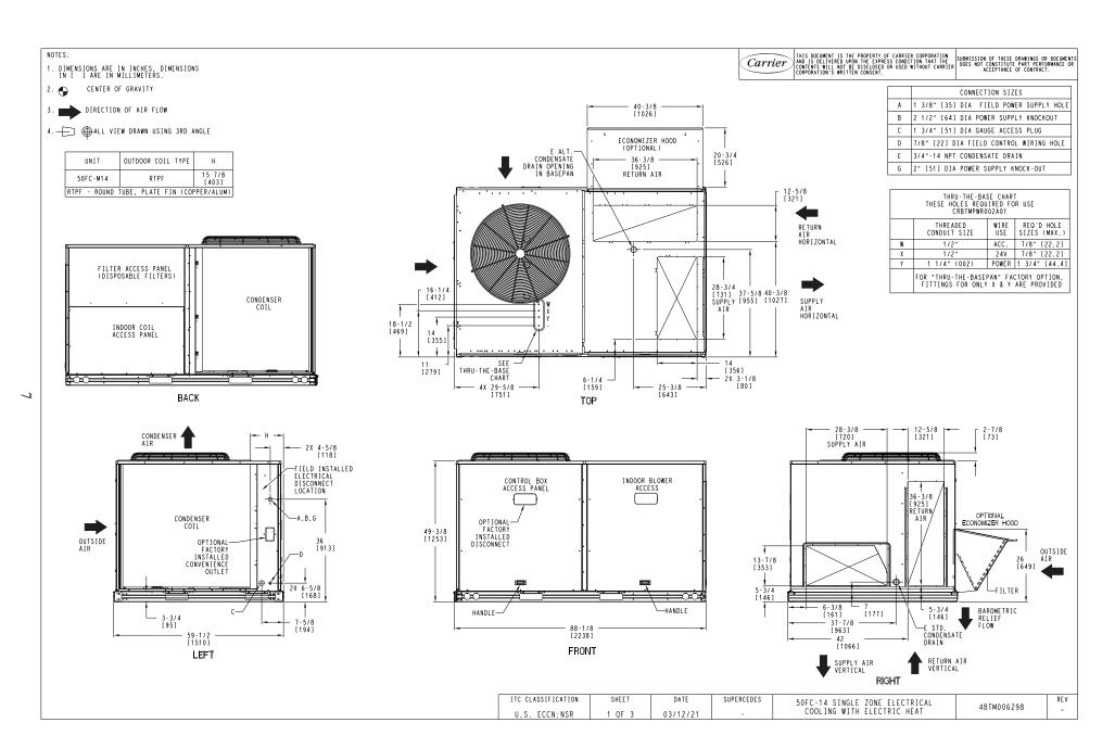
Fig. 3 — 50FC 14 Unit Dimensional Drawing
