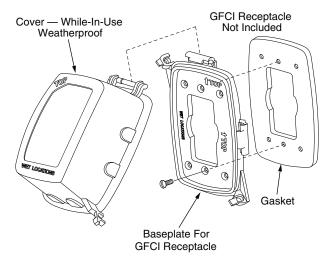
Fig. 24 — Weatherproof Cover Installation
