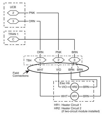
Fig. 34 — Accessory Electric Heater Control Connections
