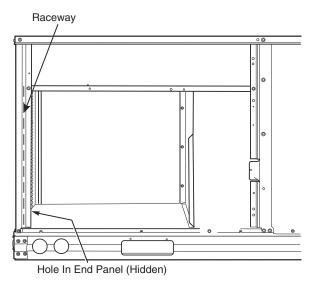
Fig. 29 — Field Control Wiring Raceway
