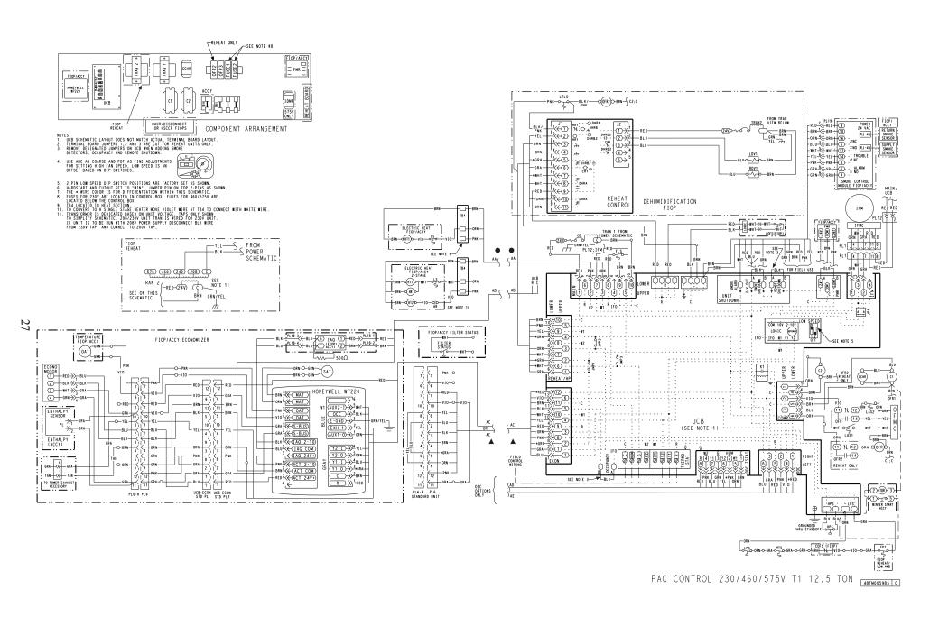
Fig. 42 — Typical Control Wiring Diagram, Electro-Mechanical with W7220 – 50FC 14, 230/460/575-3-60 Units Shown
