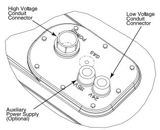
Fig. 27 — Thru-Base Connection Fittings
