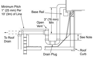
NOTE: Trap should be deep enough to offset maximum unit static difference. A 4 in. (102 mm) trap is recommended.
