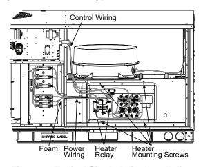
Fig. 33 — Typical Single Point Installation
