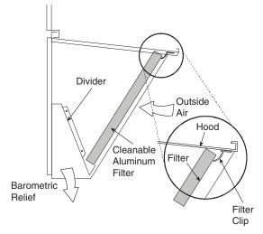
Fig. 14 — Economizer Filter Installation
