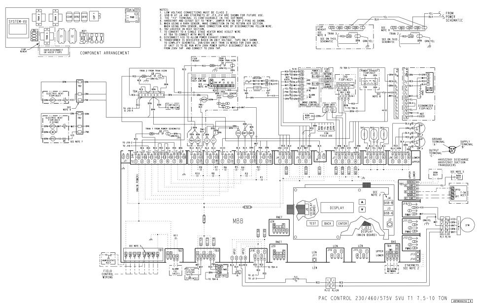
Fig. 40 — Typical Control Wiring Diagram, SystemVu™ Controller (50FC 08-12 230/460/575-3-60 Unit Shown)
