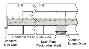
Fig. 15 — Condensate Drain Pan (Side View)
