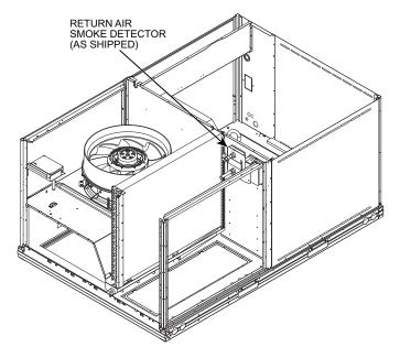
Fig. 50 — Return Air Smoke Detector, Shipping Position
