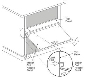
Fig. 12 — Indoor Coil Access Panel Relocation
