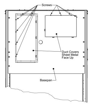
Fig. 9 — Horizontal Duct Panels In Place
