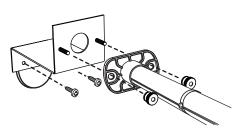
Fig. 2 Attach lamp to lamp bracked and install in desired location.
